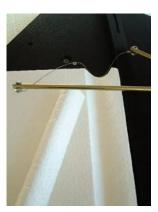
Mount the Router Blade between the two Horizontal Posts. Secure the Router Blade ends with the nuts. Move the Tool Cord connector from under the Table and clip it onto the Horizontal Post 2 that normally has no power connector. The other Horizontal Post 1 should also be connected to the Tool Cord.
