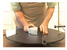
Fence closer or farther from the blade at this time. The smaller of the Traveling Fences will work for small to medium size pieces of foam. The small Fence can also be turned upside down and run along the edge of the table when cutting small pieces.
