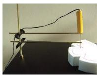
This setup allows you to make controlled samedepth engravings on the surface of a flat piece of foam.
