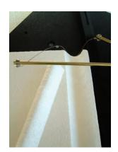
Mount the Router Blade between the two Horizontal Posts. Secure the Router Blade ends with the nuts. Move the Tool Cord connector from under the Table and clip it onto the Horizontal Post 2 that normally has no power connector. The other Horizontal Post 1 should also be connected to the Tool Cord.
