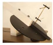
slide better. Clamp the Stationary Fence the desired distance from the Hot Wire Blade. Place the foam against the Fence and the Hot Wire Blade and turn on the power. The foam will slide through the wire, like magic.
