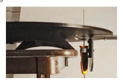
blade up or down and adjust the angle for the desired cut. As you can see, you will push the foam down onto the blade and pull it off again so you can cut holes quickly.
