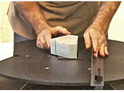
might have to adjust the Stationary Fence closer or farther from the blade at this time. The Traveling Fence will work for small to medium size pieces of foam. It can also be turned upside down and run along the edge of the table when cutting small pieces.
