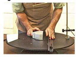
at the desired angle and distance in relation to the Blade and Stationary fence. You might have to adjust the Stationary Fence closer or farther from the blade at this time. The smaller of the Traveling Fences will work for small to medium size pieces of foam. The small Fence can also be turned upside down and run along the edge of the table when cutting small pieces.
