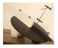
slide better. Clamp the Stationary Fence the desired distance from the Hot Wire Blade. Place the foam against the Fence and the Hot Wire Blade and turn on the power. The foam will slide through the wire, like magic.
