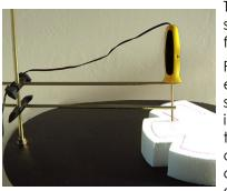
This setup allows you to make controlled same-depth engravings on the surface of a flat piece of foam.
